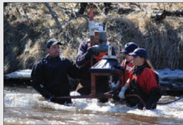
Sonar site crew deploy the DIDSON transducer into the river each spring.
