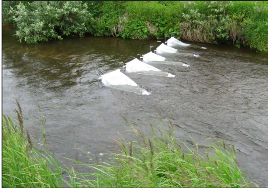
Figure 12. Driftnet configuration for macroinvertebrate sampling, South Fork Koktuli monitoring reach.
