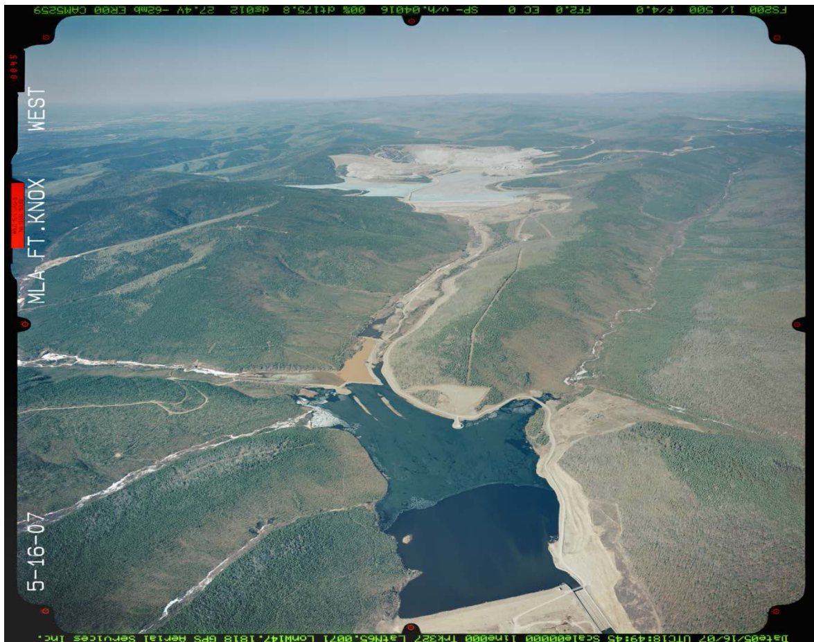
Figure 1. Aerial photograph of the Fort Knox Gold Mine water supply reservoir, tailing facility, and pit – water supply reservoir in lower part of photo and the tailing dam and impoundment in the upper Fish Creek valley, photograph provided by FGMI.
