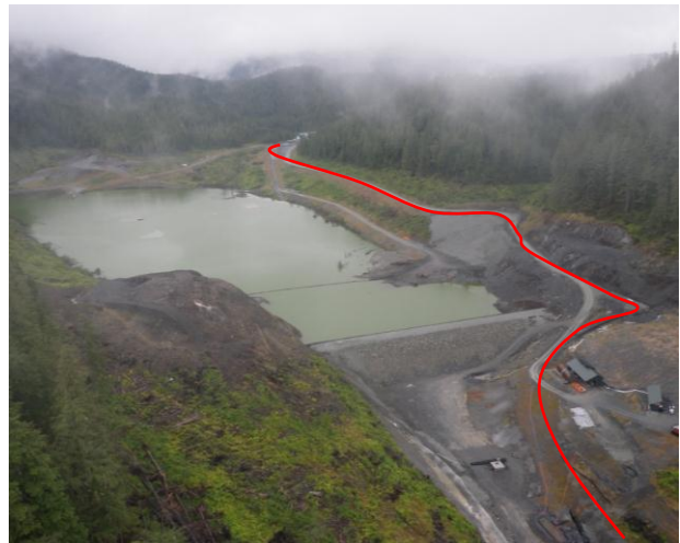
Figure 20.—Approximate diversion pipeline route.
