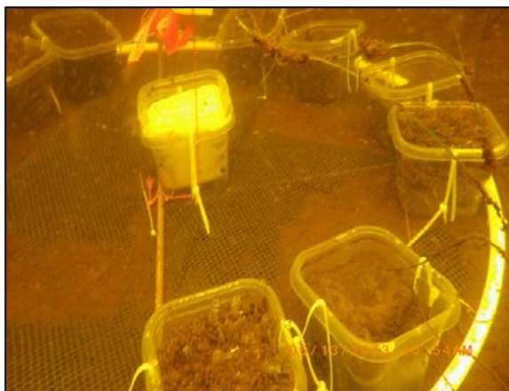
Figure 10.—Deployed array with upland soil and reference substrate trays and center sediment trap.
