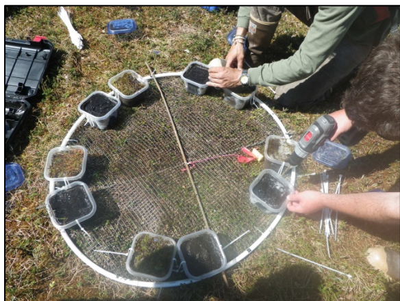
Figure 9.—Assembled PVC array with rebar and mesh support, and the paired sample trays.
