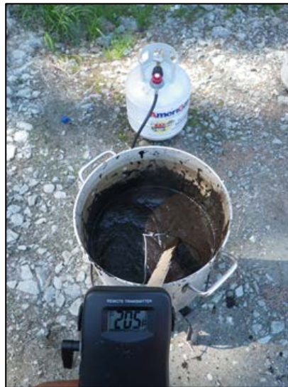
Figure 7.–Heating lakebed Upper Slate Lake substrate to eradicate insects.
