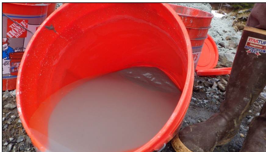
Figure 3.—Decanting supernatant water after tailings wash.
