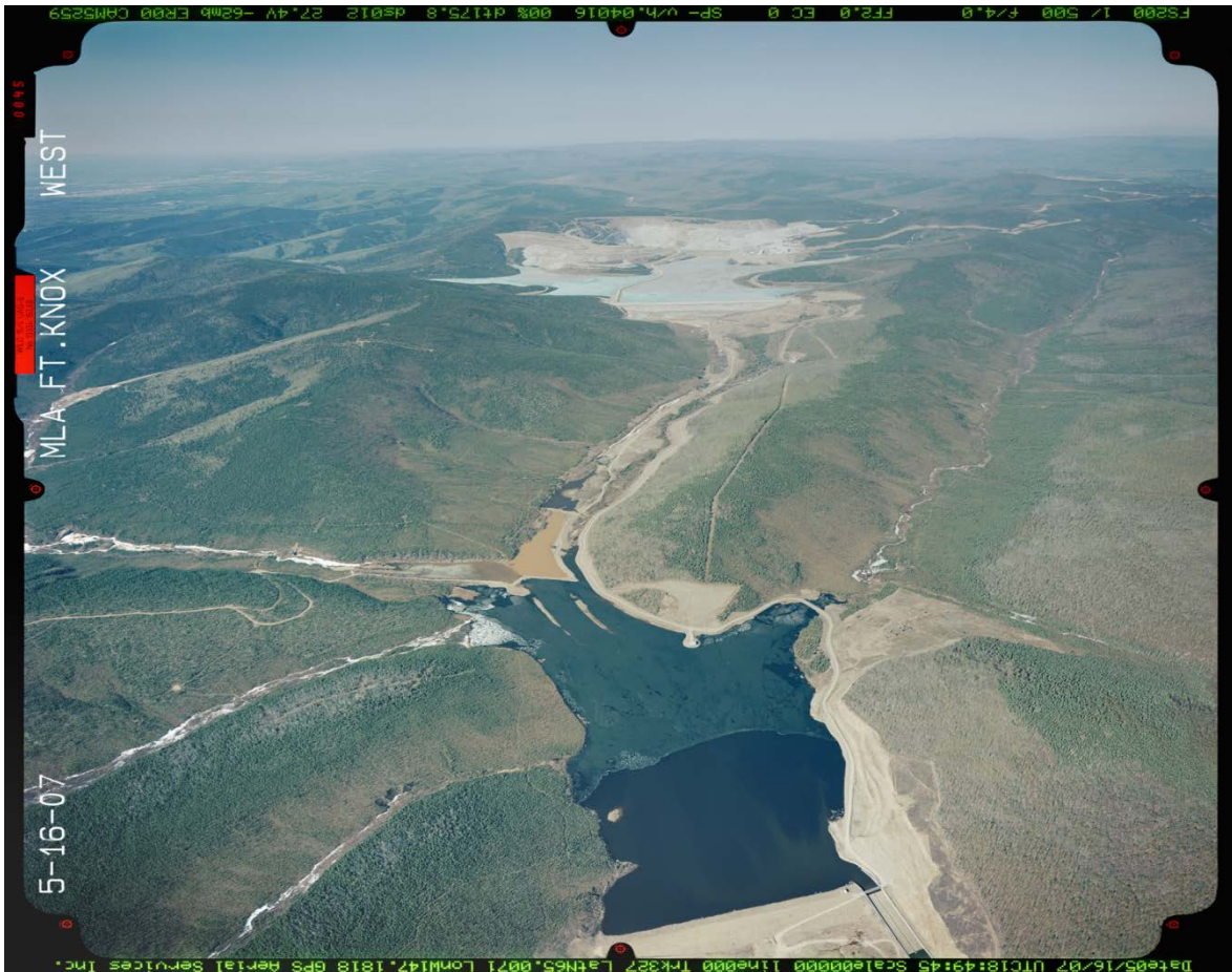
Figure 1. Aerial photograph of the Fort Knox Gold Mine WSR, tailing facility, and pit – water supply reservoir in lower part of photo and the tailing dam and impoundment in the upper Fish Creek valley, photograph provided by FGMI.
