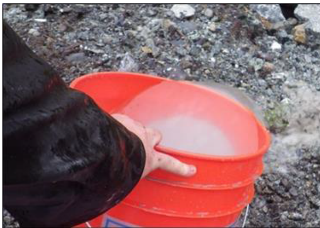
Figure 3.–Decanting supernatant water while washing the tailings.
