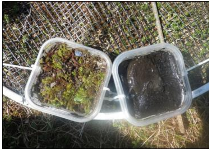
Figure 4.—Prepared upland soil (left) and reference lakebed substrate (right) sample trays.
