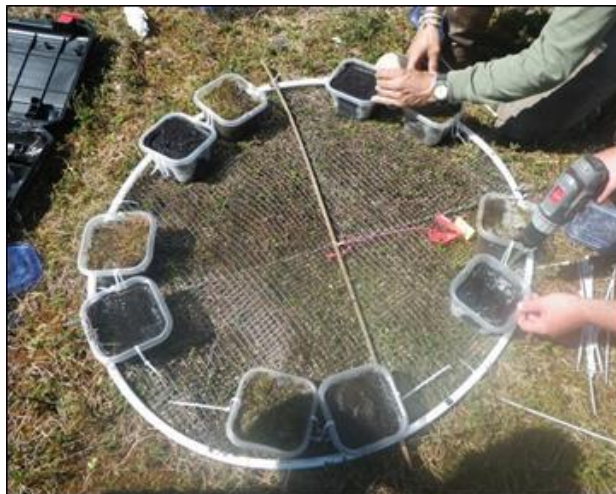
Figure 5.—Assembling an array with upland soil and reference substrate sample trays.
