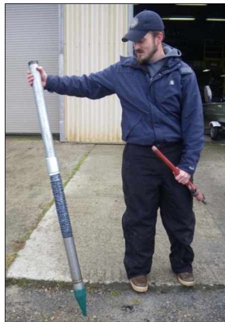
Figure 12.—Well point housing for the intragravel water quality data logger.
