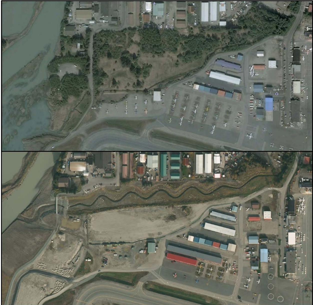
Figure 1.–Duck Creek before (top) and after (bottom) channel realignment.
