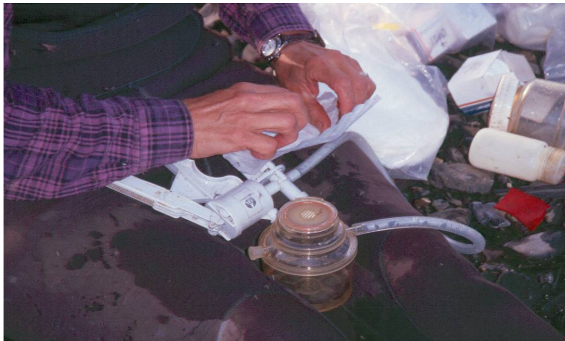
Figure 6. The folded glass fiber filter is placed in a coffee filter. The coffee filter is folded to completely cover the sample glass fiber filter.
