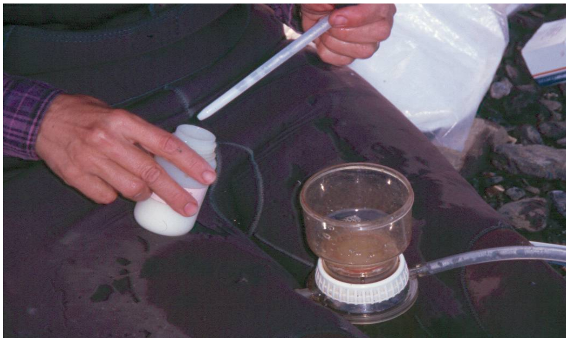
Figure 5. MgCO_3 is added to sample in the filter receptacle.
