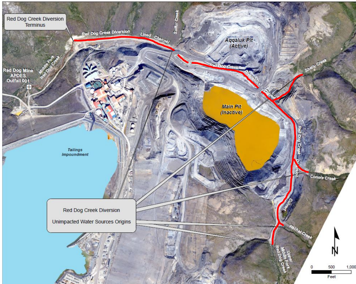
Figure 4. Clean water bypass system at the Red Dog Mine. The Red Dog Creek diversion structure (delineated by labels in the photograph and shown in red) picks up non-mining impacted waters from upstream tributaries and moves them between the Aqqaluk pit and the main pit back to the original Middle Fork Red Dog Creek streambed (flow is from right to left). 2
