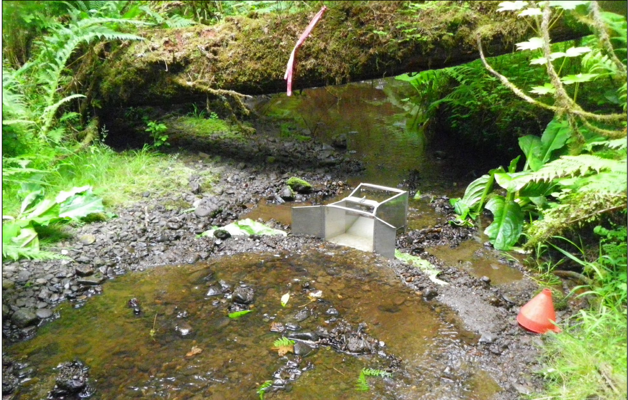
Figure 11.—Tributary Creek Site 1847; we used a Cutthroat flume to measure discharge at the lower extent of the periphyton and benthic macroinvertebrate sampling reach, July 11, 2019.
