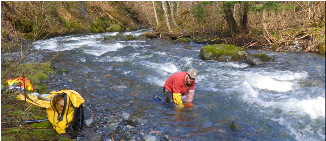
Figure 13.—Benthic macroinvertebrate sample collection in Lower Sherman Creek at SP2, May 4, 2020.
