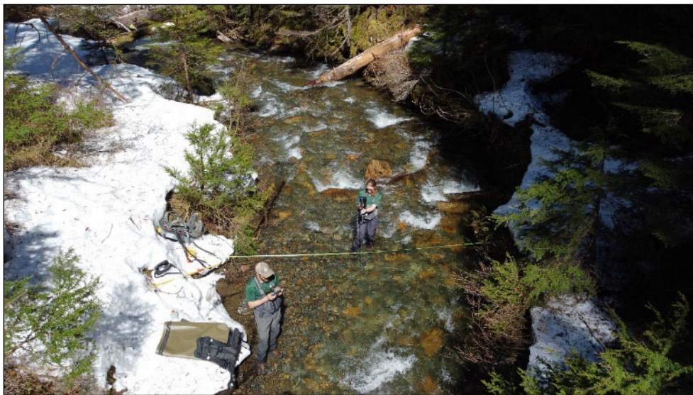
Figure 7.–Habitat Section biologists recording discharge measurement at the upstream station, 6/23/2023.
