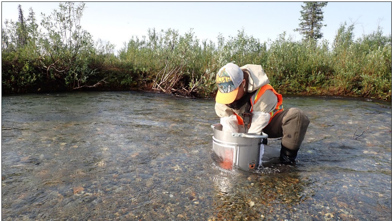
Figure 9.—Collecting invertebrate samples using a Hess sampler on Lower Subarctic Creek.
