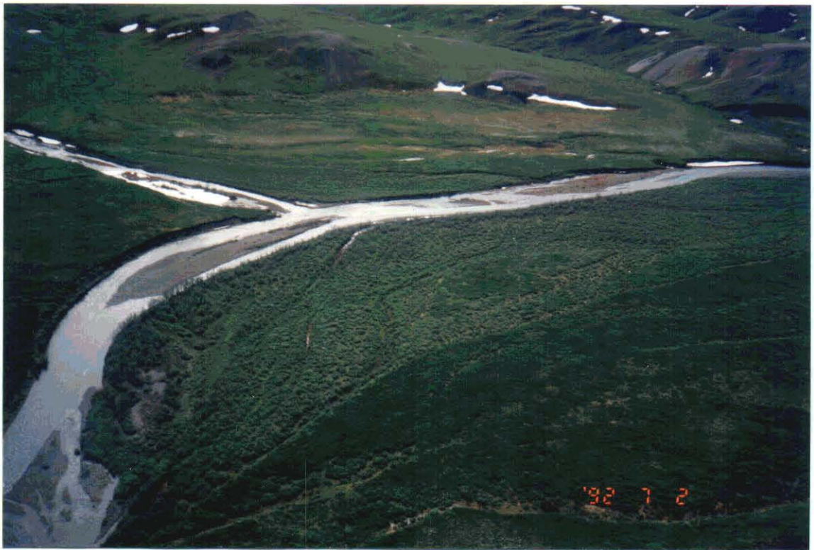
Figure 4. Rock-lined clean-water bypass ditch on right, road in middle, and dirty-water collection trench on left (top photo - July 1992). Clear water is documented at the confluence of Red Dog and Ikalukrok Creeks in July 1992 (bottom photo).
