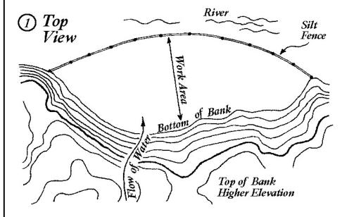
Prepare a stormwater pollution prevention plan. Set up silt fences according to terrain, soil and run-off consideration. Prevent soil migration by decreasing soil exposure, steep unvegetated slopes and construction time. Revegetate as soon as possible in the SAME SEASON.
