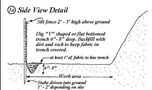
Moniter integrity of installed silt fence and remove sediment before it reaches 1/4 - 1/2 the height of the silt fence. It is especially important to moniter during and after rain and break-up events.
