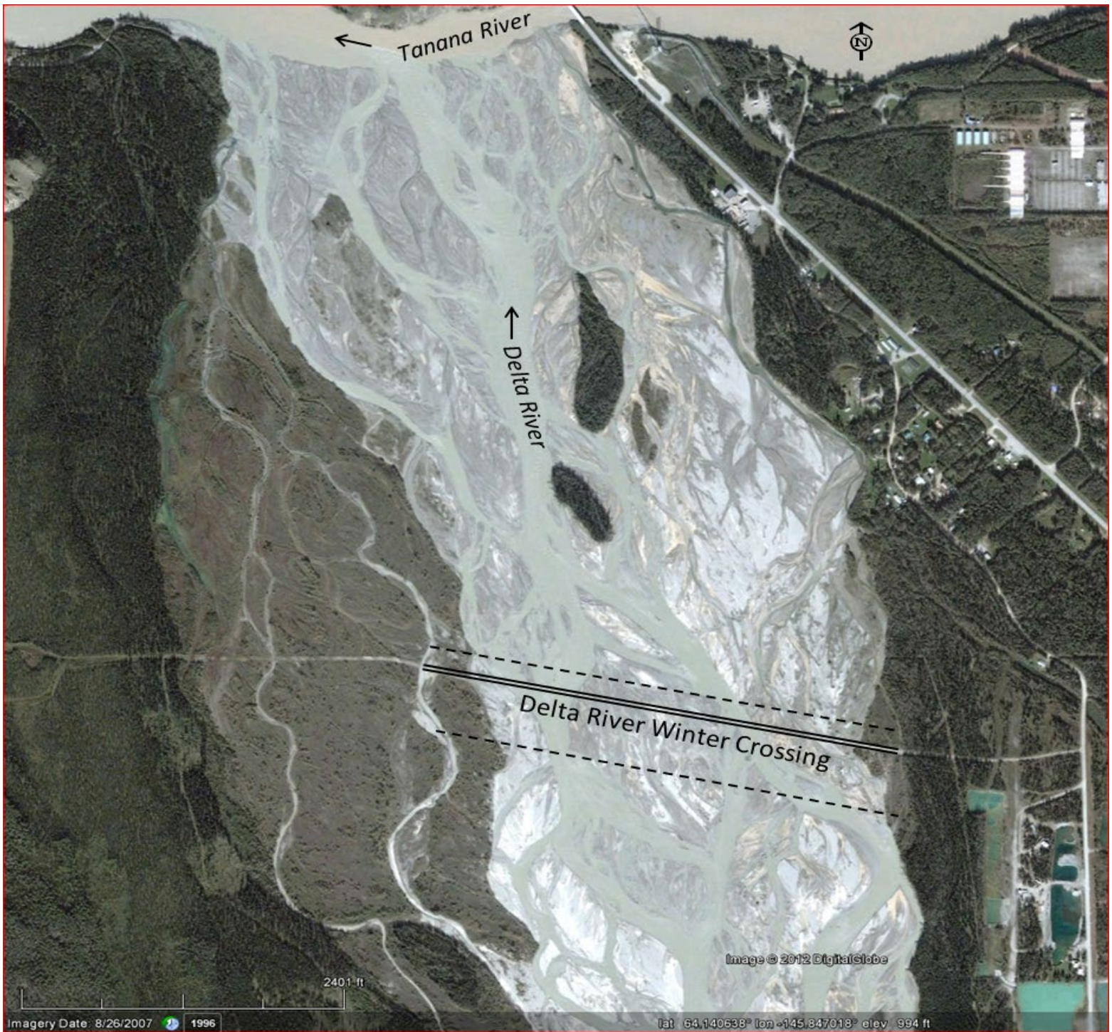
Figure 1. Lower Delta River winter vehicle crossing corridor. The double solid line is the reference line for the crossing route, and the dashed lines are the corridor boundaries.
