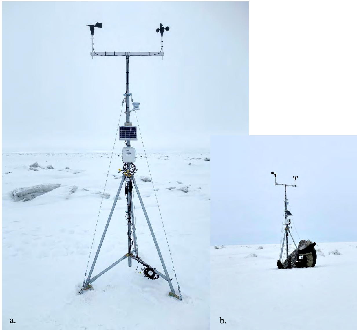
Figure 5. Meteorological (MET) station deployed on the sea ice in our study area (a). Data were downloaded from the MET station onto a laptop computer weekly (b).
